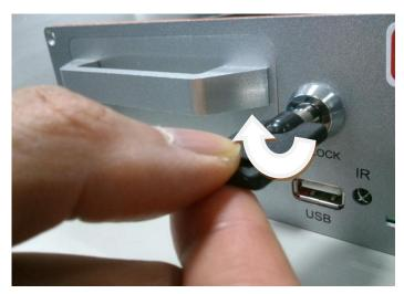
After you installed the SSD, please put the rack back into the mobile DVR, tighten the two front screws and lock the rack. If the lock is not correctly done, the system won't be started up and the power led will flash.
