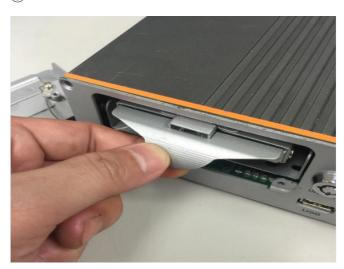
④ Turn the rack over to install SSD. Please take note of the direction and tighten SSD up by the four screws.
