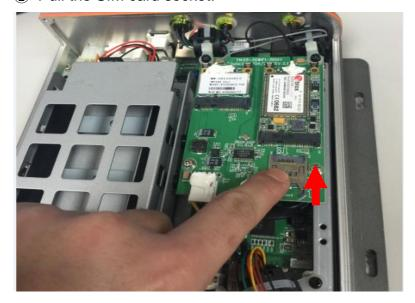
③ Insert the SIM card with its gold contact facing down and as below shown.
